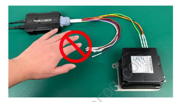
When some airbag ecu are being repaired, the CG70 will read the original EEPROM data, which must be saved for subsequent maintenance.
