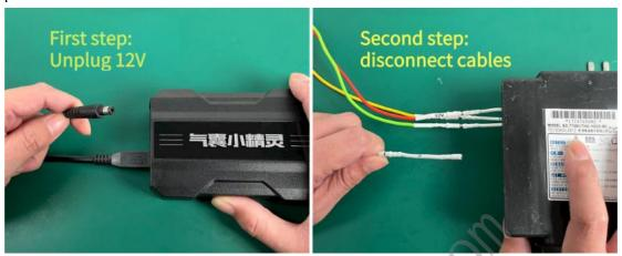
Do not move the airbag module after CG70 has been repaired successfully. let it stand for five minutes after the power is turned off. The purpose is to discharge the capacitor to prevent damage to components.
