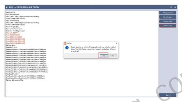
Click "Restore Data" to write the ECU data. Please make sure the data is backed up before writing. The restored data will overwrite the current ECU data. The data can be the data of the current ECU or other ECUs of the same type.
