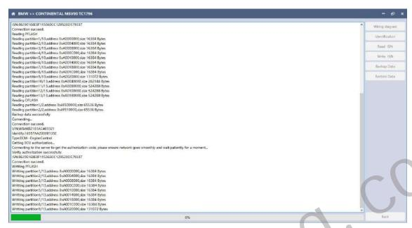
Note: During the process of data recovery, it is strictly forbidden to disconnect the device power or disconnect the device, otherwise it may cause damage to the ECU; if the software is unexpectedly shut down or the computer is shut down or crashed unexpectedly during the process of data recovery, please do not disconnect the device power or device Connect for 15 minutes, and the device can complete data recovery independently.
